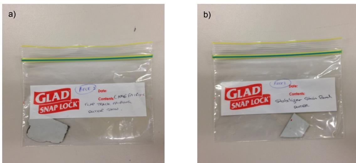
Fig. 1: a. Item 2. Right wing No. 7 Flap Track and b. Item 3. Right Horizontal stabiliser panel, Outer Fairing, Outer Skin.
