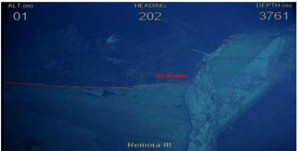
Figure 4.17: Shipwreck #4 – starboard bow damage
