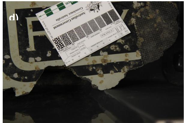
Figure 1 Overview images of Item 4 (Engine Nose Cowl); a) the external side of Item 4 indicating evidence of cementing structures; b) internal side of Item 4; c and d) close up of bottom external side of item 4
