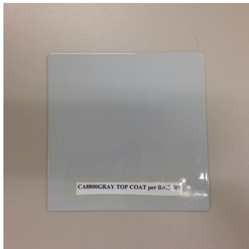
*Fig. 3: Item 3. CA8800GRAY TOP COAT per BAC 707 (from control sample)*
