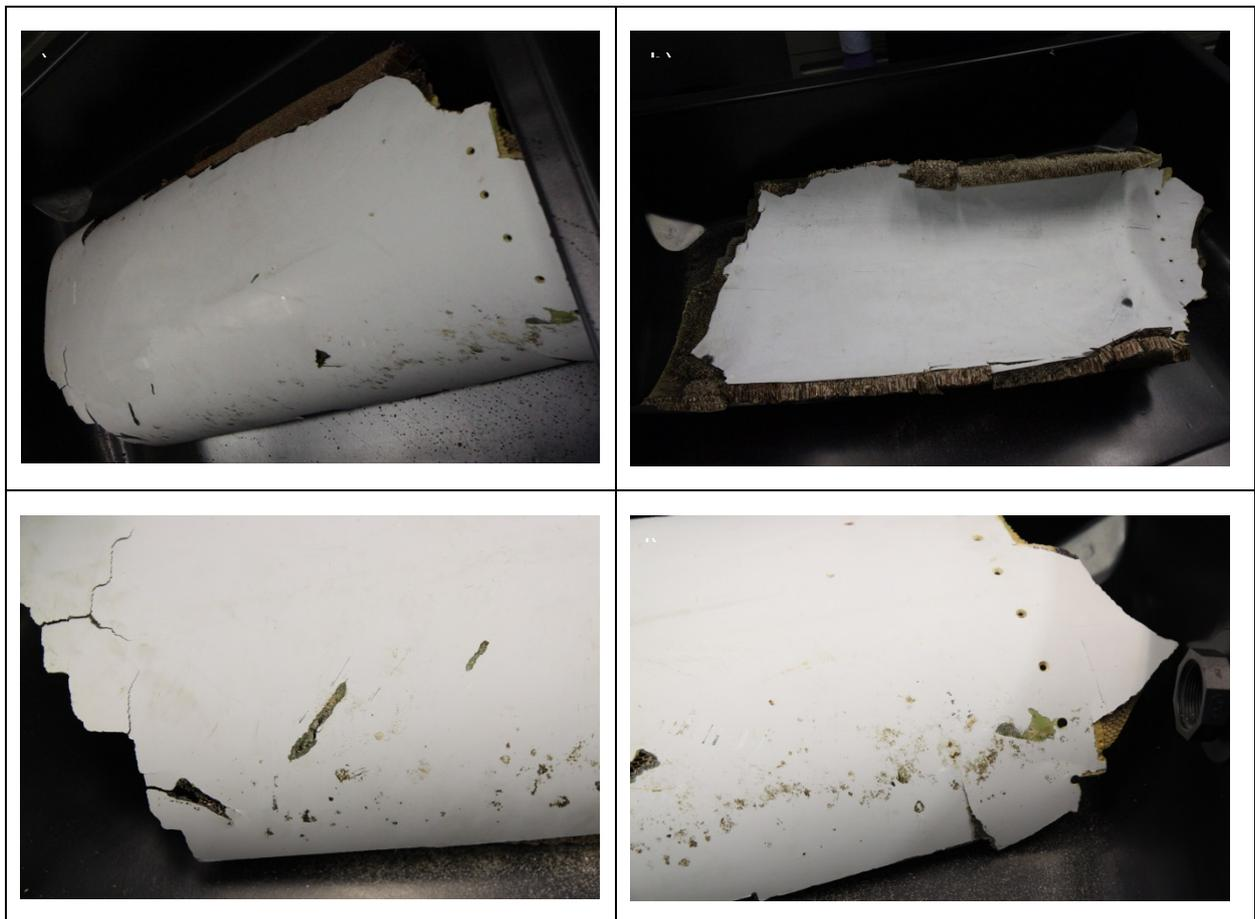
Figure 1 – Overview images of Item 2 (Right wing No. 7 flap track fairing); a) the external side of Item 2; b) internal side of Item 2; c) close up of bottom external side of Item 2; d) close up of possible remnants of barnacle cement.
