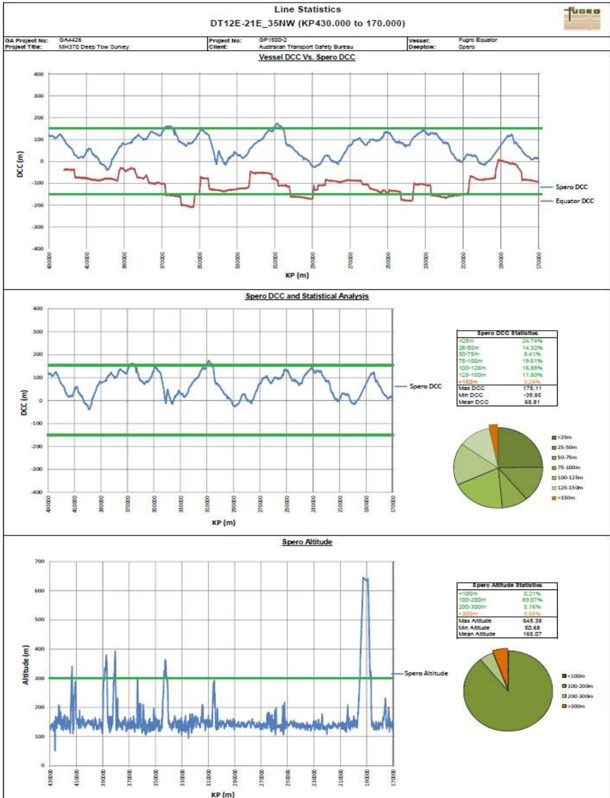
**Figure 3.2: Example line statistics showing Distance Cross Course (DCC) and Altitude at KP values**
