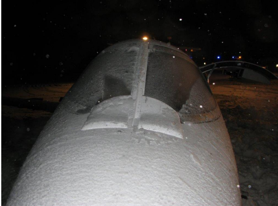
Figure 3. Photograph of a Learjet 35A with ice-covered windscreen (NTSB case number ANC12IA024).
